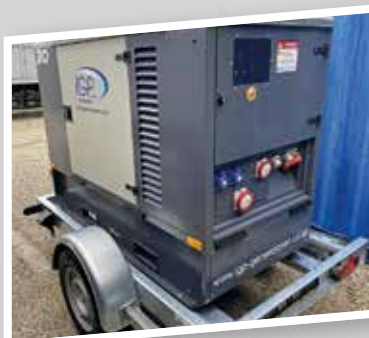
Mobiles Aggregat 30 kVA
